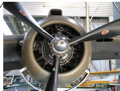
Afb 1. 14 cilinder (2x7) ster
